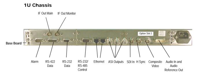
Figure 1.10: E5714 (1U) Rear Panel Component Parts and Connectors
